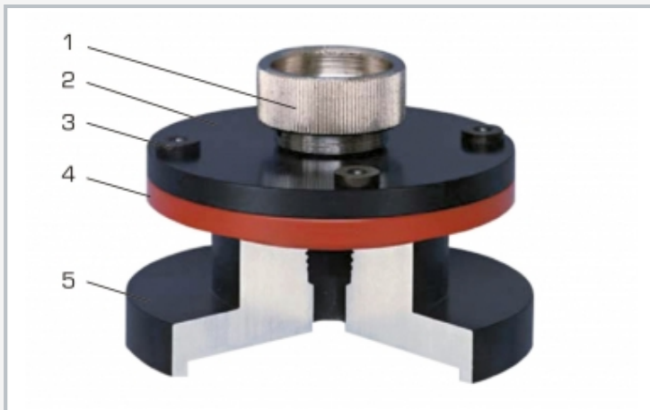
Assembled drilling jig with workpiece: 1 fastening screw, 2 drill plate, 3 drill bush, 4 workpiece (bearing cap), 5 base
